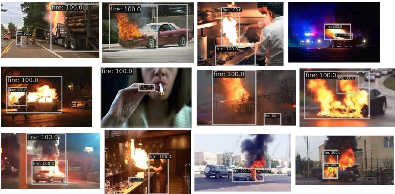
Figure IV.9: YOLO-CLIP zero-shot detection of all COCO categories + 'fire' category but only the n=2 objects classifications with highest certainty
