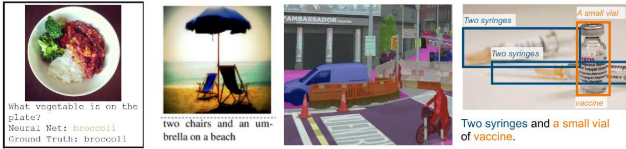
Figure II.4: Task examples for VLM models. From left to right: Visual Question Answering (VQA), Visual Captioning (VC), Semantic Segmentation (SS), Grounding Referring Expressions (GRE)
